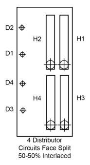
FIGURE 92 - STACKED COIL DESIGN (STANDARD)
