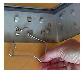
FIGURE 112 - CORRECTLY INSTALLED LATCH PIN (P/N 026-35778-007)
