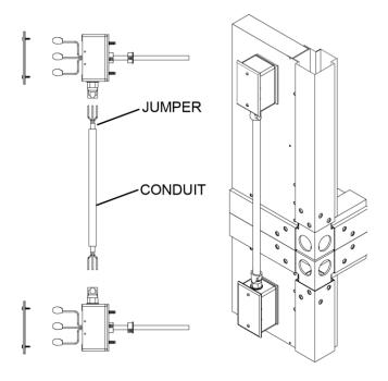
FIGURE 45 - LIGHTS TIER TRANSITION DRAWING
