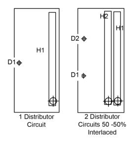
FIGURE 90 - NON-STACKED COIL DESIGN (STANDARD)
