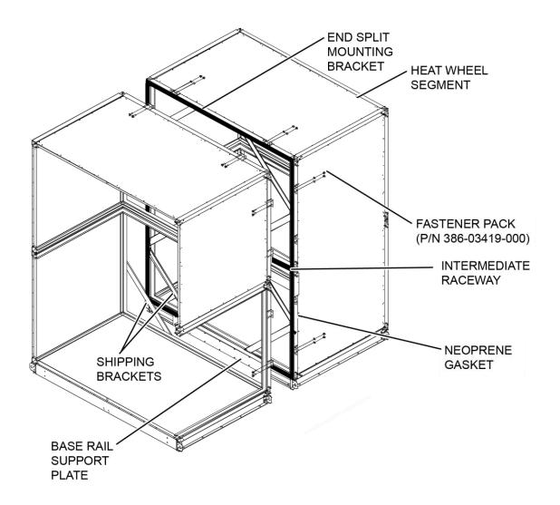
FIGURE 46 - ASSEMBLING THE END CHANNEL SHIPPING SPLIT WITH ENERGY RECOVERY WHEEL
