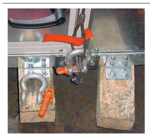
FIGURE 12 – PROPER LIFTING WITH SHACKLE AT LIFTING LUG
