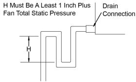
Top Of Trap Must Be Equal To Or Lower Than Bottom Of Unit Drain Connection
