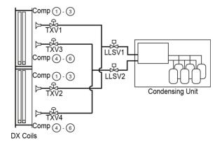
FIGURE 98 - SIX COMPRESSOR UNIT
