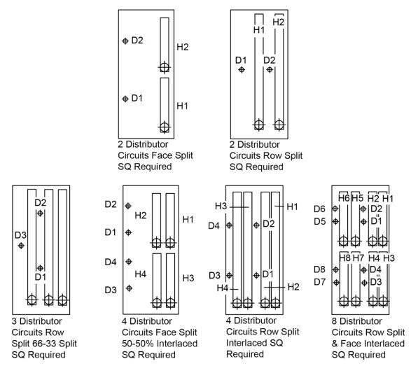
FIGURE 91 - NON-STACKED COIL DESIGN (SPECIAL QUOTE)
