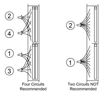
FIGURE 94 - STACKED COIL CIRCUITING
