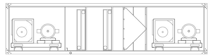
FIGURE 1 - CUTAWAY OF ESL SHOWING SEGMENTED CONSTRUCTION
