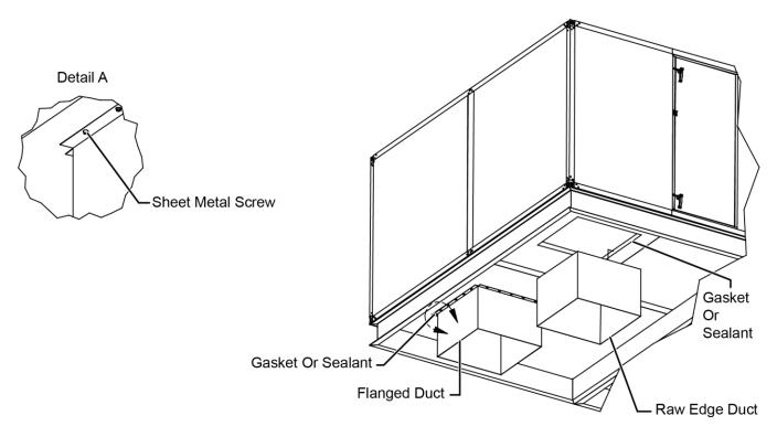
FIGURE 104 - DUCT ARRANGEMENT FOR FLANGE AND RAW EDGE DUCTS
