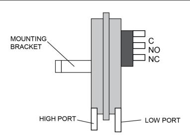
FIGURE 71 - AIR FLOW SWITCH CONNECTIONS
