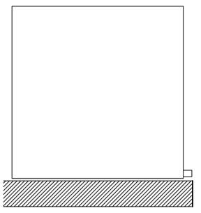
FIGURE 14 - NO BASE RAIL – HOUSEKEEPING PAD REQUIRED TO ACCOMODATE TRAP HEIGHT
