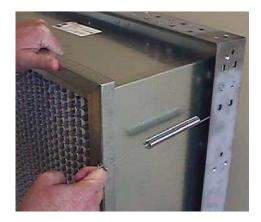
FIGURE 117 - SPRING LATCH PULLED AND FASTENED IN FILTER HOLE
