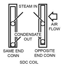
FIGURE 76 - FACTORY COIL CONNECTIONS
