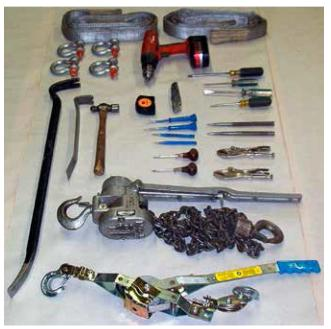
FIGURE 18 - TOOLS NEEDED TO ASSEMBLE SHIPPING SPLITS
