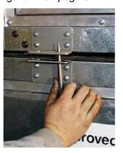
FIGURE 44 - GUIDE BRACKETS TOGETHER
