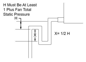
FIGURE 100 - TRAP DETAIL FOR DRAIN PAN IN NEGATIVE ENVIRONMENT (DRAW THROUGH)
