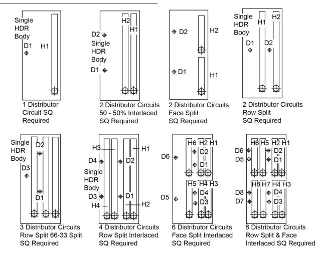
FIGURE 93 - STACK COIL DESIGNS (SPECIAL QUOTE)
