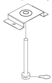
FIGURE 49 - DAMPER SHAFT EXTENSION KIT (P/N 026-33715-002)
