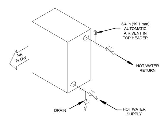
FIGURE 86 - HOT WATER PIPING FOR IFB
