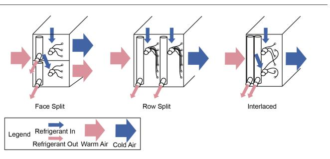
FIGURE 89 - DX COIL CIRCUITING TYPES
