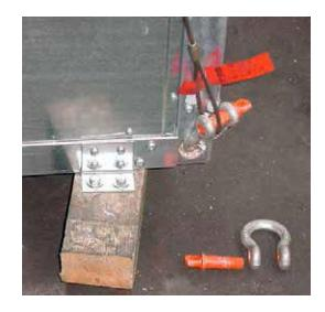
FIGURE 11 - PROPER LIFTING WITH SHACKLE WITH CORNER CONNECTOR CORNERS
