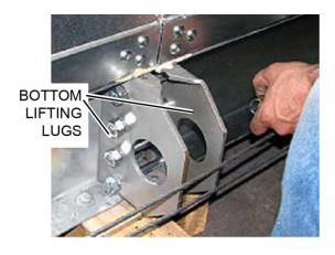
FIGURE 38 - FASTEN BOTTOM LIFTING LUGS
