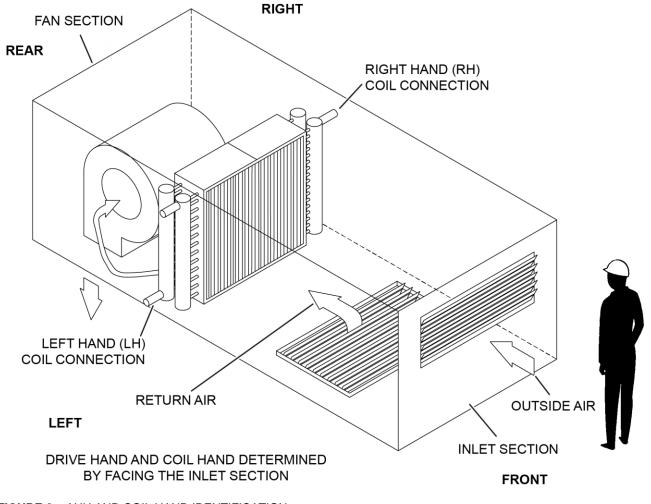
FIGURE 2 - AHU AND COIL HAND IDENTIFICATION
