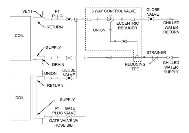
FIGURE 79 - CHILLED WATER COIL CONNECTIONS EXAMPLE - (NOT FOR CONSTRUCTION)
