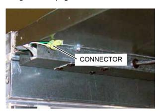
FIGURE 34 - ELECTRICAL CONNECTOR (NOT CONNECTED)
