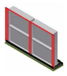
FIGURE 78 - SPLIT COIL - OPPOSITE SIDE CONNECTIONS
