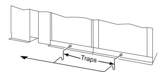
FIGURE 102 - COMBINING DRAIN LINES
