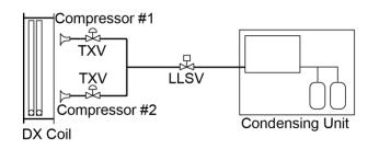
FIGURE 96 - TWO COIL CIRCUIT PER REFRIGERANT CIRCUIT
