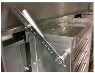
FIGURE 51 - COUNTERBALANCE UNLOCKED FOR START-UP
