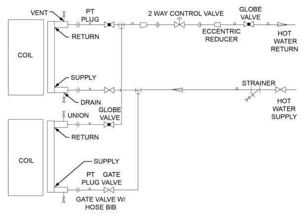
FIGURE 80 - HOT WATER PIPING WITH 2 WAY VALVE EXAMPLE (NOT FOR CONSTRUCTION)
