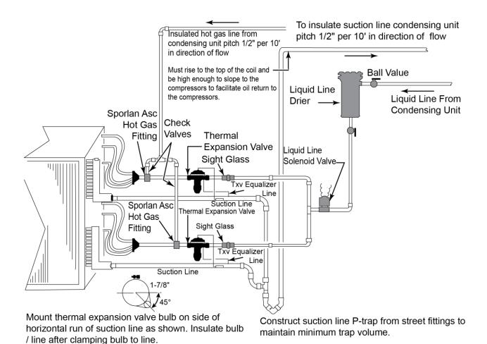
FIGURE 88 - TYPICAL PIPING AND SUNDRIES AT THE DX COIL
