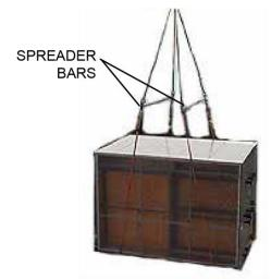
FIGURE 9 – RECOMMENDED LIFTING WITH FOUR CORNER POINTS
