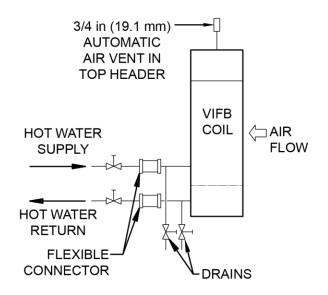
**FIGURE 85 -** HOT WATER PIPING SCHEMATIC FOR 2-ROW COIL VIFB
