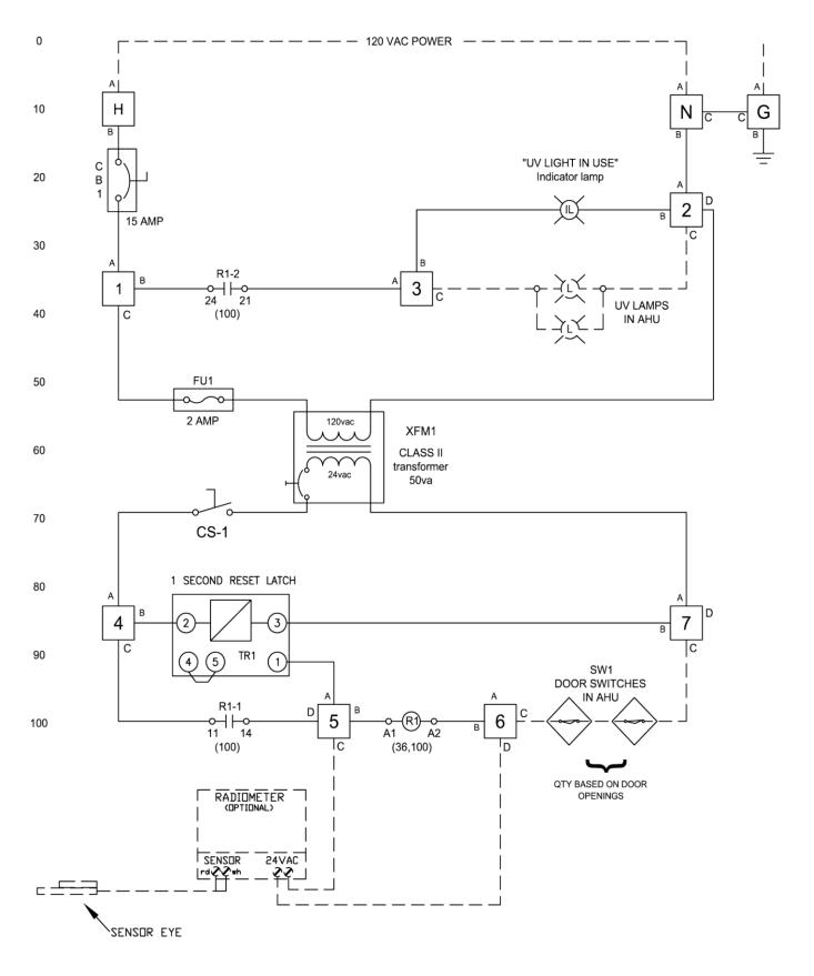
FIGURE 55 - UV CONTROL PANEL WIRING (8 AMPS)
