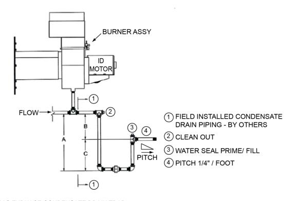
FIGURE 59 - GAS FURNACE CONDENSATE DRAIN TRAP
