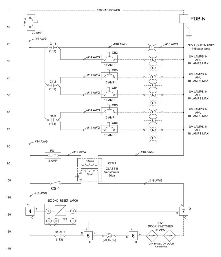
FIGURE 56 – UV CONTROL PANEL WIRING (GREATER THAN 8 AMPS)
