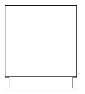
FIGURE 15 - NO HOUSEKEEPING PAD – BASE RAIL REQUIRED TO ACCOMODATE TRAP HEIGHT
