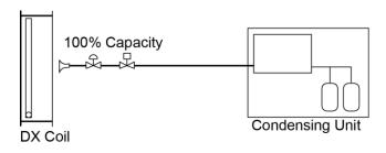
FIGURE 95 - ONE COIL CIRCUIT PER REFRIGER-ANT CIRCUIT
