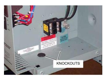
FIGURE 73 - SUPPLY POWER KNOCKOUTS
