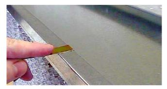
FIGURE 120 - INSTALLING PRE-FILTER LATCH
