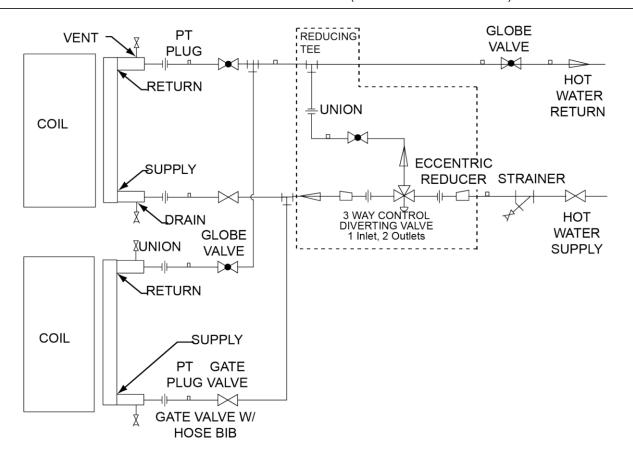
FIGURE 81 - HOT WATER PIPING WITH DIVERTING VALVE EXAMPLE (NOT FOR CONSTRUCTION)
