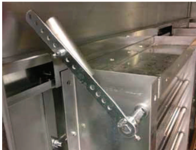
FIGURE 5 - COUNTERBALANCE UNLOCKED FOR START-UP
