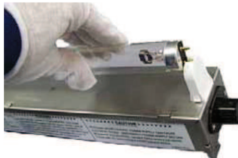
FIGURE 53 - INSTALLING V-MOD LAMP
