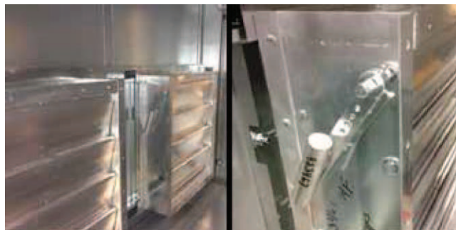
FIGURE 4 - COUNTERBALANCE LOCKED INTO PLACE FOR SHIPPING
