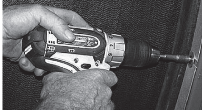
FIGURE 66 - LOOSEN SCREWS BEFORE ADJUSTING SEALS
