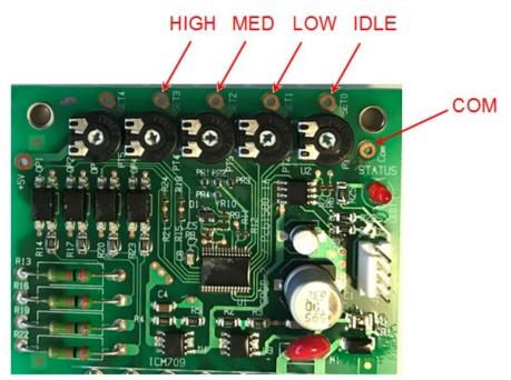
Figure 3 - Select PWM Test Points (front)
