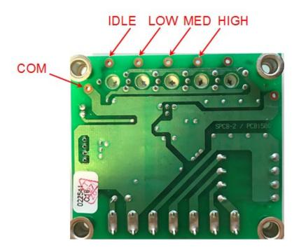
Figure 4 - Select PWM Test Points (back)
