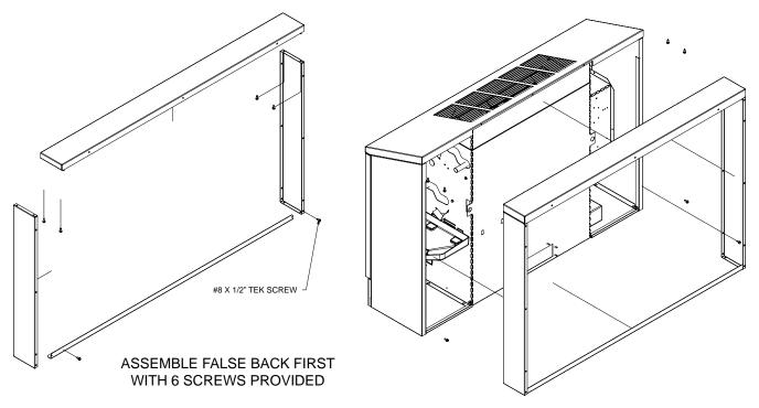
ATTACH FALSE BACK TO UNIT WITH REMAINDER OF SCREWS PROVIDED
