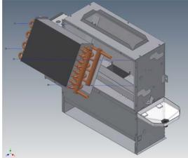
Remove screws to replace coil.
