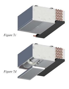
Figure 7a-7d: Filter removal
