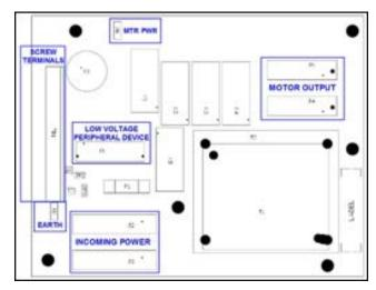
Figure F.2 – Connector layout
