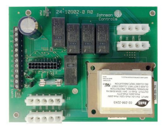
Figure F.1: Fan Relay Board (FRBii)
