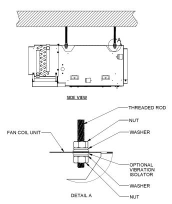
Figure 1: Typical ceiling installation
