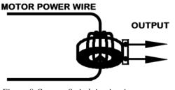
Figure 9 Current Switch in circuit
