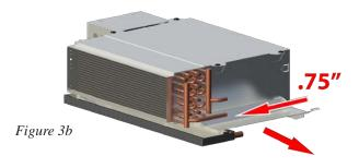
Figure 3a-3b: Typical auxiliary drain pan removal
