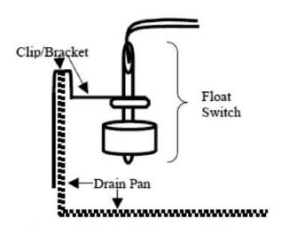
Figure 15b: Drain pan float switch diagram
