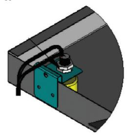
Figure 15a: Drain pan float switch installed
