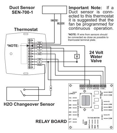
2-Pipe, Low Voltage Valve, H2O Changeover Sensor
