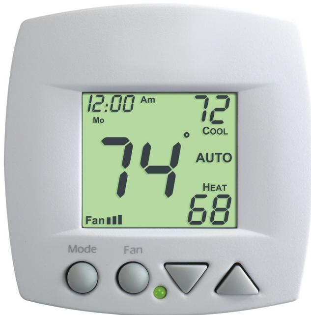
The T701DFN Non-programmable and T701DFP Programmable thermostat controllers provide control of two or four-pipe fan coils. These thermostat controllers provide on/off; three speeds of fan control, and dry contact unoccupied control. They are designed as standalone devices for use in commercial buildings such as schools and hotels. The thermostats provide the user access to parameters such as system mode, fan mode, and temperature setpoints.
