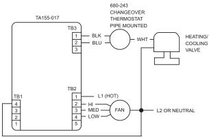
Figure-5 Typical 2-Pipe Heating/Cooling Fan Runs with System Switch On or Off.
