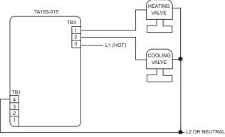
Figure-4 Typical 4-Pipe Heating/Cooling. No Fan Connections.
