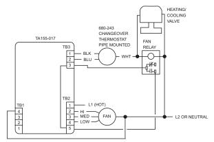
Figure-6 Typical 2-Pipe Heating/Cooling Fan Cycles with Demand for Heating or Cooling. With System Switch Off, Fan is Off.
