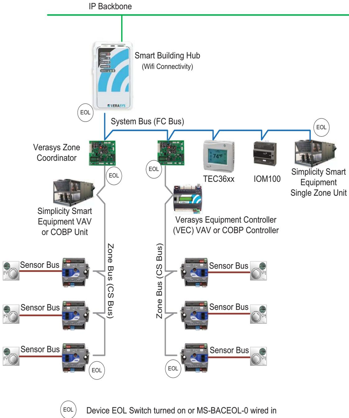
Note the Smart Building Hub does not have an EOL switch. To terminate a device that does not have an EOL use an MS-BACEOL-0 and wire it to the end of the trunk or reposition the device to where it is not end of line.
