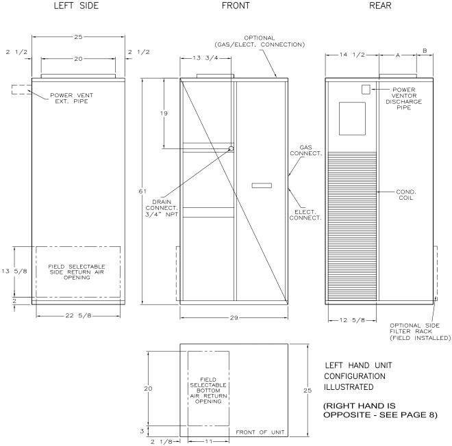
IMPORTANT: POWER VENTOR DISCHARGE PIPE MUST TERMINATE 1"-1 1/4" FROM EXTERIOR GRILLE/LOUVRE. MATERIALS FROM
