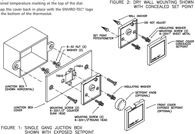
NOTE: The temperature setpoint adjustment on the ETST4H thermostat is reversed from the older (ETSTAT) series thermostats. When using the 600 Series IOM manual in conjunction with the ETST4H, the direction of rotation of this setpoint should be reversed from the direction stated in manual's instructions.
