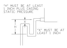
**FIGURE 4B**Trap detail for positive cabinet static pressure
