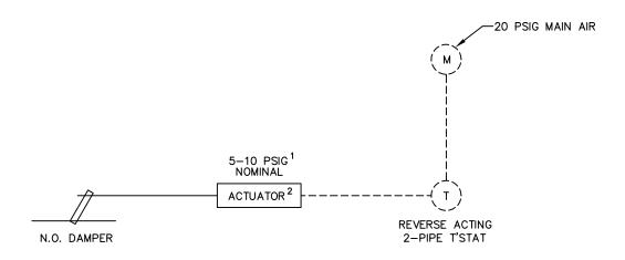
NOMINAL SPRING RANGE IS FOR UNLOADED OPERATION. ACTUAL LOADED RANGE WILL VARY AND IS DEPENDENT ON MECHANICAL STOPS (IF UTILIZED). THIS SEQUENCE IS NOT RECOMMENDED FOR APPLICATIONS REQUIRING DIRECT SEQUENCING WITH OTHER CONTROL DEVICES. (i.e. DDC/ PNEUMATIC CONTROL DEVICES BY OTHERS)
