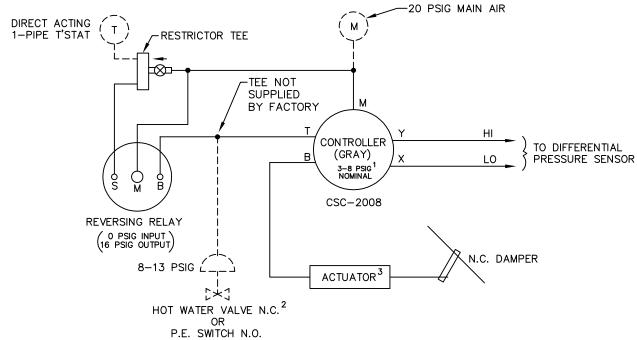
CONTROLLER REQUIRES FIELD CALIBRATION AND SET UP UNLESS OTHERWISE SPECIFIED. CONTROLLER RESET RANGE WILL VARY WITH AIR FLOW LIMITS.
