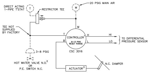
CONTROLLER REQUIRES FIELD CALIBRATION AND SET UP UNLESS OTHERWISE SPECIFIED. IF FACTORY CALIBRATION OPTION IS USED, THE RESET SPAN AND STARTPOINT WILL BE ADJUSTED AS SHOWN ABOVE UNLESS OTHERWISE SPECIFIED.
