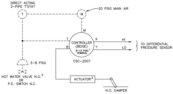
CONTROLLER REQUIRES FIELD CALIBRATION AND SET UP UNLESS OTHERWISE SPECIFIED. CONTROLLER RESET RANGE WILL VARY WITH AIR FLOW LIMITS.
