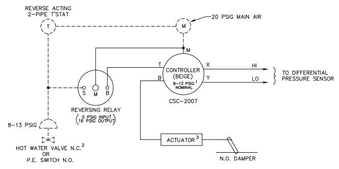
CONTROLLER REQUIRES FIELD CALIBRATION AND SET UP UNLESS OTHERWISE SPECIFIED. CONTROLLER RESET RANGE WILL VARY WITH AIR FLOW LIMITS.
