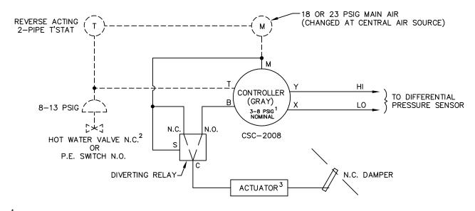
CONTROLLER REQUIRES FIELD CALIBRATION AND SET UP UNLESS OTHERWISE SPECIFIED. IF FACTORY CALIBRATION OPTION IS USED, THE RESET SPAN AND STARTPOINT WILL BE ADJUSTED AS SHOWN ABOVE UNLESS OTHERWISE SPECIFIED.
